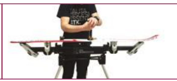
3 | Vise mode for mounting and maintenance of bindings
